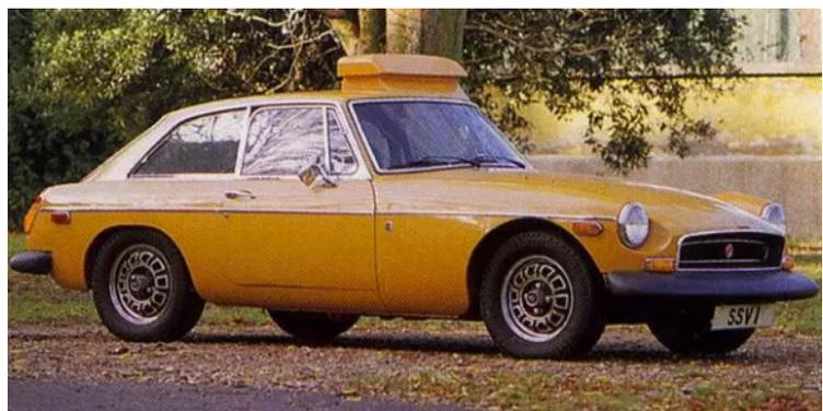
The SSV1 was prepared by the development team at Abingdon in 1972 to demonstrate that even small cars were capable of being modified for optimum safety. This MGB GT-based car featured a wealth of innovative features, including airbags (which worked in combination with passive seat-belts), anti-lock brakes, self-levelling suspension, impact-absorbing side-panels and a rather curious roof-mounted rearview mirror which afforded the driver a 120-degree field of vision.
