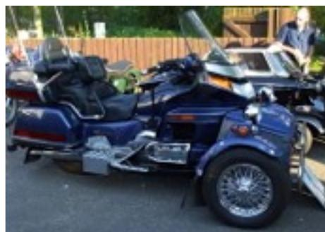
I then covered in the steering box with a "Mini" bonnet which I cut and welded to suit the necessary size. I hinged it at the front - pull a bonnet catch and a "V.W. Golf" gas strut opens the bonnet. Brakes are all linked to my foot pedal. As it is triked the law requires a parking brake, this was made from a 70's "Honda CB100"
