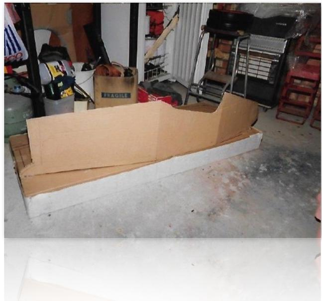
So with that idea in mind we set about designing cardboard templates and full-size drawings on pieces of card. Then I made plywood formers to shape the galvanised sheet metal that I had chosen to form the body panels out of. I thought the galvanised sheet steel may keep the rust away to give it a longer life.
