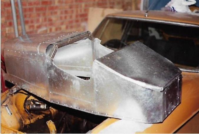
The chassis was welded up using one inch square mild steel tube with the body being pop riveted in position, then the hard part trying to find wheels and tyres to fit. In those days, without the likes of eBay, it took some time to come up with the wheels. Eventually I found two brand new wheel barrow wheels (not quite what I wanted but needs must), then I had to order the other two and wait weeks for them to arrive.
