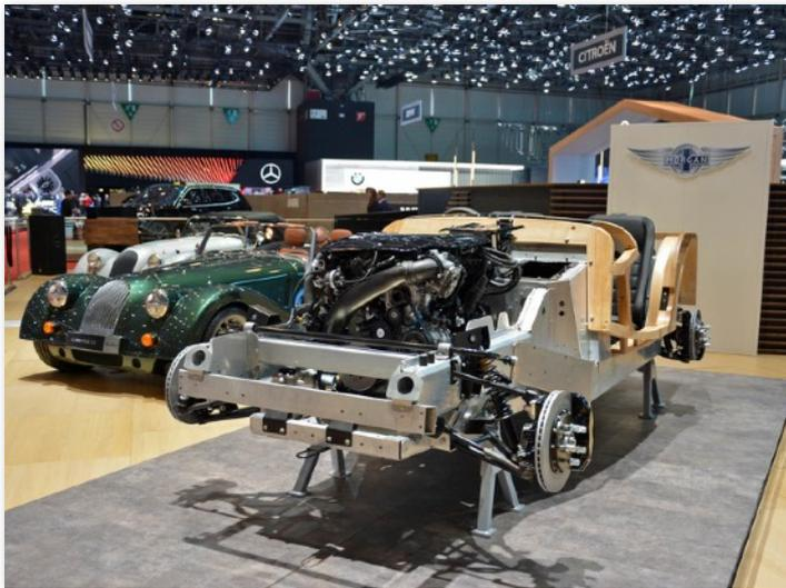
architecture. The all-new CX-Generation bonded aluminium platform has been designed and developed in-house and is introduced with intention for use in future premium Morgan models throughout the next decade.
