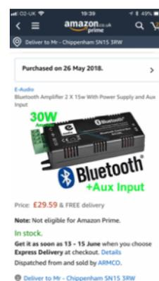
The power cable just needs snipping, there are two wires, one is plain and the Earth has white dashes. Connect the dashed cable to an earth and the other to a 12v positive feed. The Green plug that you can see in the picture comes out and you can attach your speaker cables before plugging it back in. Then all you need to do is hide it up somewhere with cable ties. Then just pair the device and hey presto...
