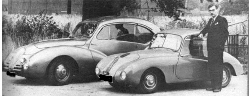
produced in Coventry around an ash frame fabricated by a local boat-builder.
