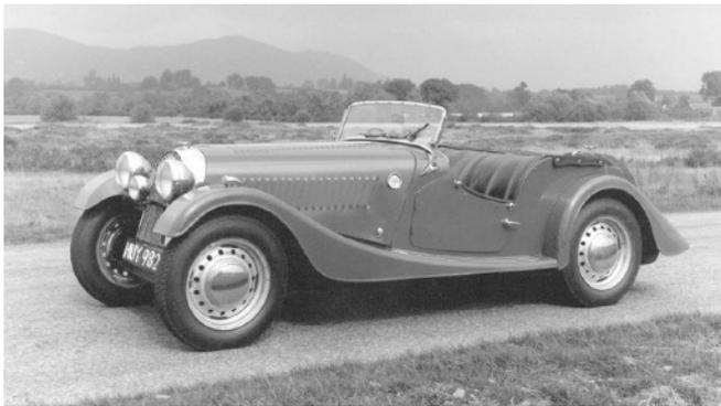
Coincident with the demise of the Plus 4, 2020 marks the 70th anniversary of the Plus 4. The Plus 4 at its introduction in 1950, was fitted with a 2088cc Standard Vanguard engine installed on a strengthened 4/4 chassis with a wheelbase lengthened by 4 in (102 mm). Hydraulic brakes, at first all drum, were fitted for the first time on a Morgan.
