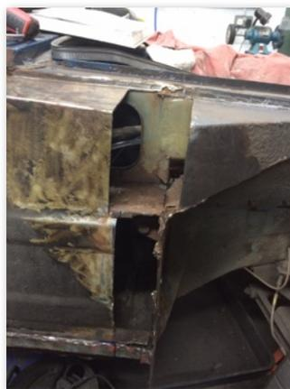
work on the offside wing which had some rather draughty rust holes in it. I managed to patch and lead load the deep damage and use Ultimate filler in
