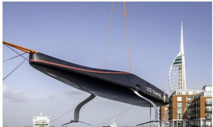
The 2021 America's Cup boats are high tech, 75 feet long, carbon fibre monohulls. Flying on hydrofoils that lift the entire keelless, six-tonne monohull and 11-man crew clear of the water. Many questioned whether it was technically possible to balance a single-hulled boat of this size with no keel on just two hydrofoils.
