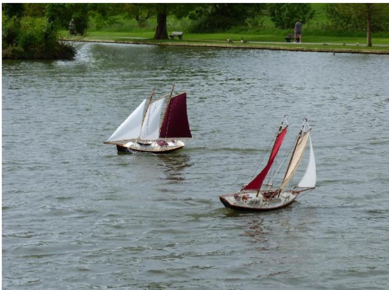
a boat in Mexico! A club friend and I built them to 90% of the original model size too enable them too fit into our cars..The sails and rudder are radio controlled through servos. The sail servo is a winch in the back of the boat with a return pulley at the front. The sails are sheeted in and out on a closed loop of cord below deck..
