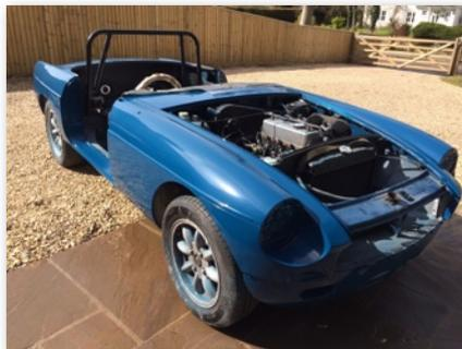
etch primed (yellow), primer filler applied(white), flatted back and then a guide coat is used (black). This is sanded back and any low spots are obvious as the black paint is left behind. These small defects are filled with acrylic stopper. Flatted back again then second coat primer filler
